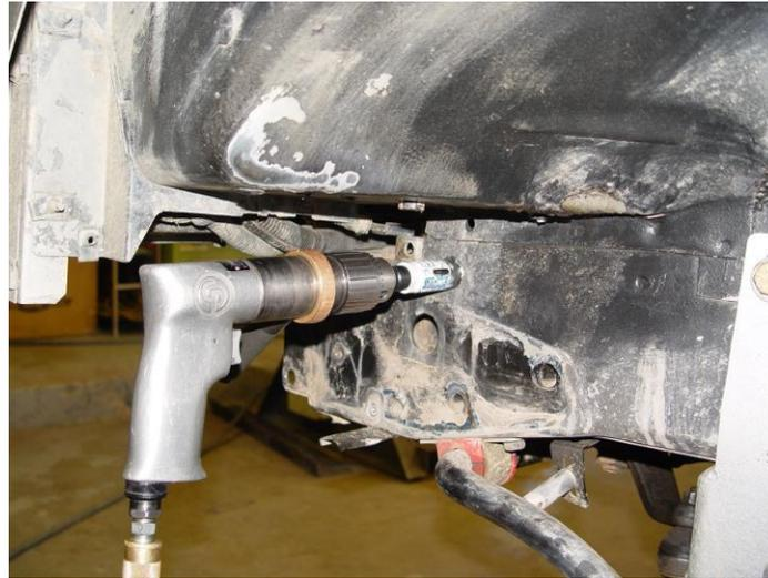
Continue to cut into the unibody to the depth of the whole saw as shown below. Ensure that the cut is level and square
