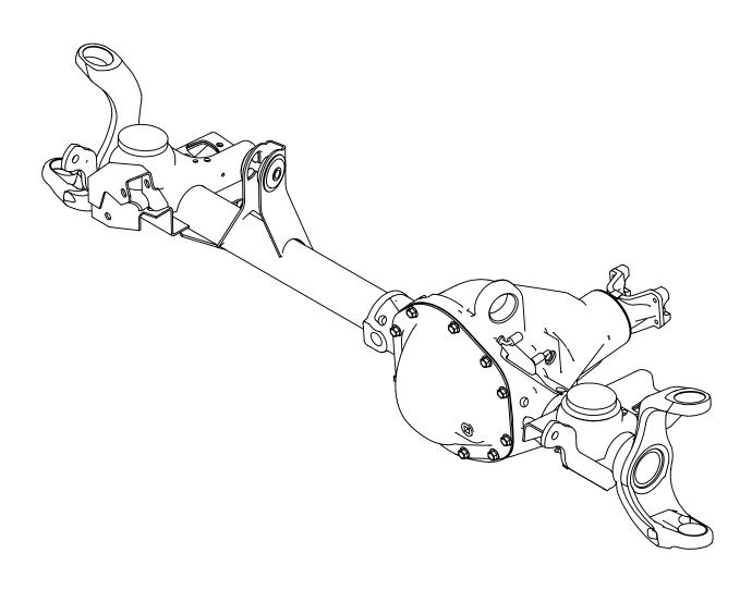
Step 3: Trim driver side upper control arm mount so that you have 2 posts that fit into the 2 cut outs in the top of the bridge about an 1/8" below the top of the bridge. Step 4: Bevel the bridge where the axle tube goes so it clears the welds
