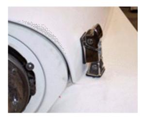
Two sets of gaskets are provided with this Hood Catch Kit. The CJ requires the tapered gaskets as shown above. The YJ gaskets are flat and straight.
