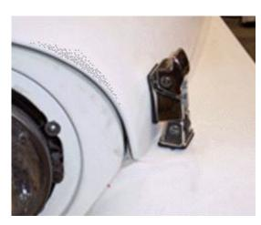
Two sets of gaskets are provided with this Hood Catch Kit. The CJ requires the tapered gaskets as shown above. The YJ gaskets are flat and straight.
