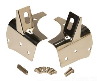
Remove the five bolts on the upper portion of the windshield hinge. Place the Light Bracket over the upper hinge and align the holes. Using the Stainless bolts provided start all five bolts then tighten evenly.
