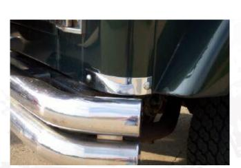
Place the rear corner guard in place and align the bottom edge of the guard with the body tub. Mark the two mounting holes with a magic marker. Center punch the mark, then drill with a small drill bit. Re-drill the holes using an 11/32" drill bit. Bolt the corner guards in place using the stainless steel bolts provided.
